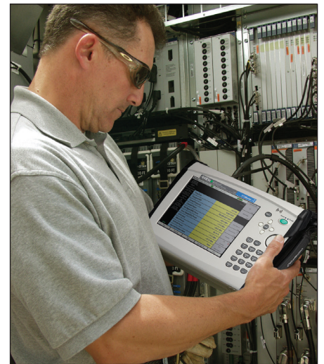
Figure 4. Technician examining spectrum at BTS location
